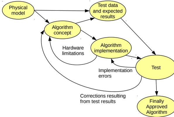
Fig. 5. The process of development and testing of the algorithm.
