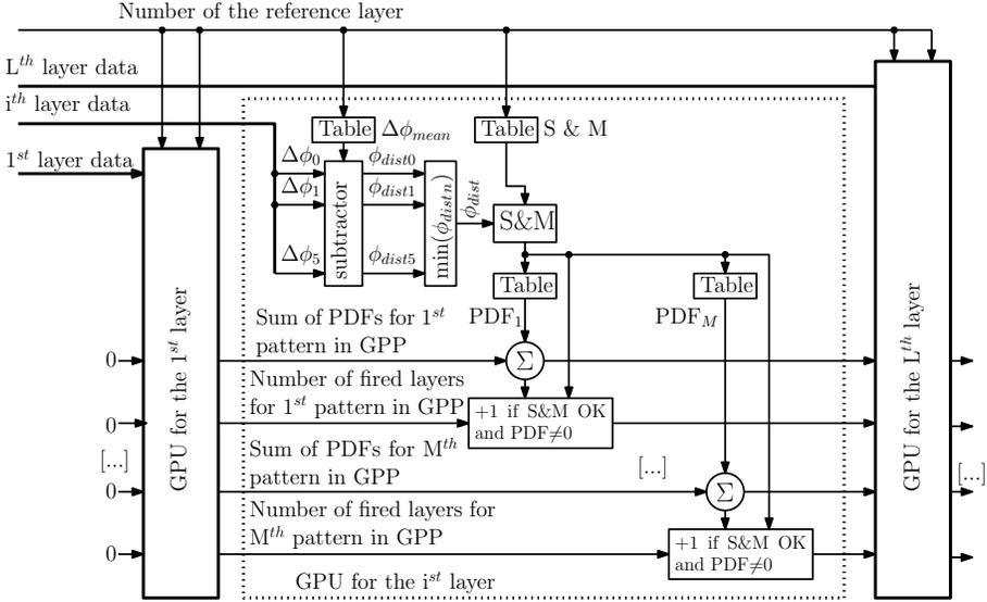
Fig. 4. Implementation of the single GPP handling  $M$  patterns. The Golden Pattern Unit (GPU) is the block which analyses hits in a single layer.  $L$  is the number of layers,  $M$  is the number of patterns handled in the GPP. “S&M” (shift and mask) are the blocks used to scale  $\Delta\phi$  depending on the PDF distribution width.
