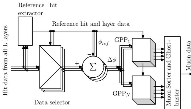
Fig. 3. Block diagram of the OMTF implementation.
