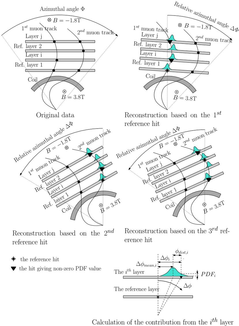
Fig. 2. The principle of operation of the OMTF algorithm. The event contains hits generated by two muons. Three reference hits were available. One of them starts the reconstruction of the track of the first muon. Two others lead to the reconstruction of the track of the second muon. The Ghostbuster algorithm should filter out the repeated detection of the second muon, so that only two muons are reported.
