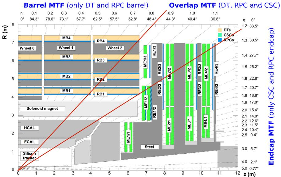
Fig. 1. The longitudinal, schematic view of the quarter of CMS detector. The muon detectors RPC (denoted as RB and RE), CSC (ME) and DT (MB) are marked. In addition, the approximate segmentation into barrel, overlap and endcap partitions is shown [3].
