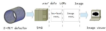
Fig. 1. Scheme of the data flow in the PET image reconstruction. The raw data collected by the Data Acquisition System (DAQ) is then processed by the low-level reconstruction module (low-level reco.) and results in the set of reconstructed lines of response (LORs), which are then sent to the image reconstruction module (Image reco.). The final image can be visualized by the dedicated image viewer or can be exported to DICOM format.
