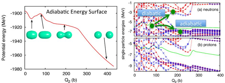
Fig. 1. (Color on-line) Left: Adiabatic potential energy curve obtained for the case of compact symmetric fission in  $^{258}\text{Fm}$ . The corresponding neutron and proton single-particle energies are shown in the right part. See Refs. [4, 5] for details. The two extreme cases of adiabatic and diabatic motions are illustrated close to level crossing.
