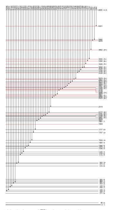
Fig. 5. Partial level schemes of  $^{210}$ Bi obtained by cold-neutron capture, showing primary decay transitions only. Newly found states are marked in gray/red [23].
