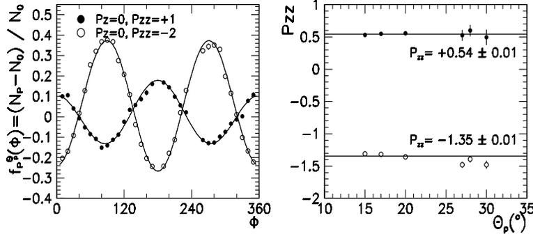
Fig. 1. Left: ratios  $f_P^{\theta_p}(\phi)$  for two pure tensor beam polarization states (nominal polarizations shown in the panel), for one chosen proton polar angle  $\theta_p = 17^\circ \pm 0.5^\circ$ ; Right: tensor polarizations  $P_{zz}$  obtained for the same two states at several angles  $\theta_p$ , with the resulting mean values.
