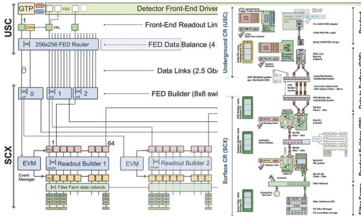
Fig. 14. The general CMS Trigger scheme (top). The DAQ system (bottom) is made of 8 independent systems (slices). Each slice consists of 64 RUs, a  $64 \times 64$  EVB and 64 BUs and associated filter units. A slice can read up to 12.5 kHz.
