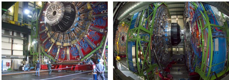
Fig. 4. CMS assembly process: YE1 (left) equipped with the muons chambers and calorimeters sliding on the floor towards YB3 (right).
