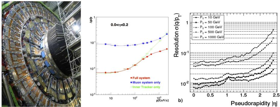
Fig. 9. Endcap disk equipped with muon chambers (left). Performance of the CMS muon system (right).
