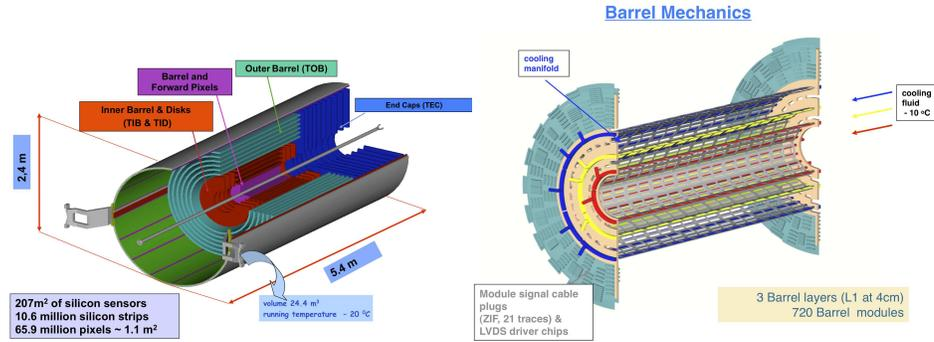
Fig. 12. Silicon tracker design (left). The barrel mechanics for the pixel detector (right).
