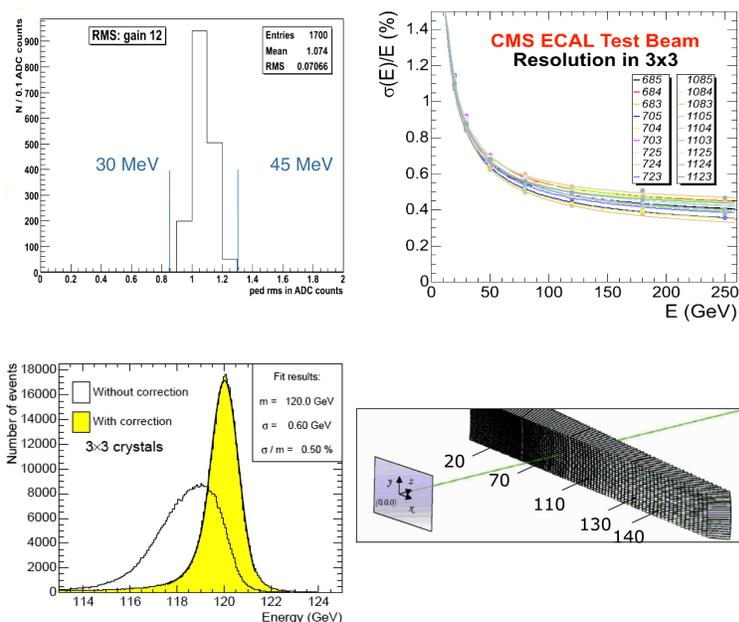
Fig. 11. Performance of the ECAL. The achieved electronics noise (40 MeV per channel) and the resolution for a  $3 \times 3$  crystal matrix (top). The corrected energy measurement for a widely illuminated SM area (bottom). The achieved resolution for 120 GeV electrons was measured to be 0.5%.
