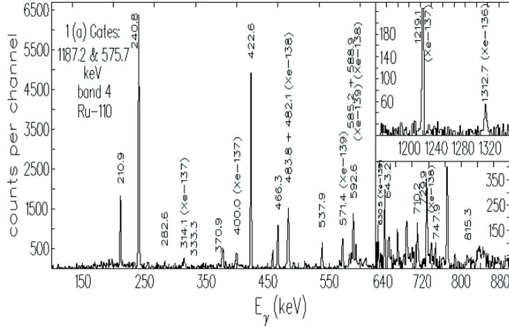
Fig. 3. Coincidence spectrum double-gated on 1187.2 and 575.7 keV ( $6^+ - 4^+$  in ground band) transitions in  $^{110}\text{Ru}$ .
