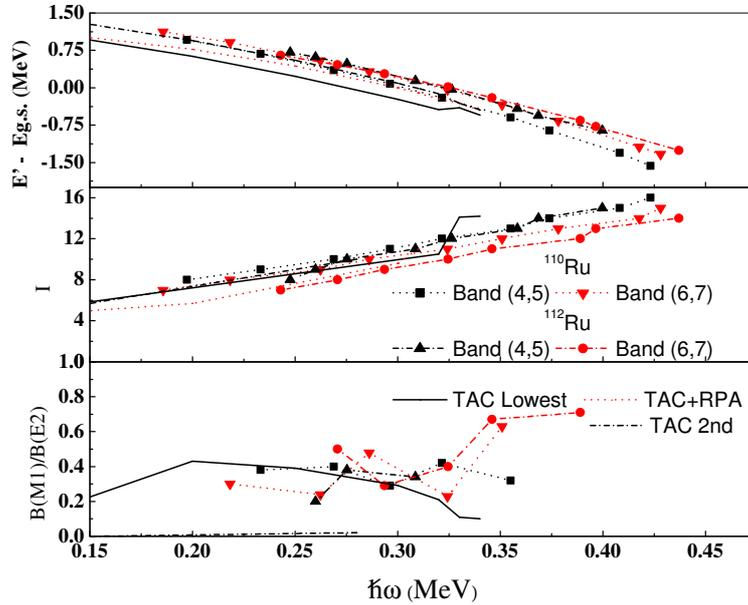
Fig. 7. Energy in the rotating frame (upper panel), angular momentum (middle panel) and  $B(M1)/B(E2)$  in-band values of the negative parity bands in  $^{110,112}\text{Ru}$  as a function of rotational frequency. Within the present approach both are equal and given by the TAC calculations.
