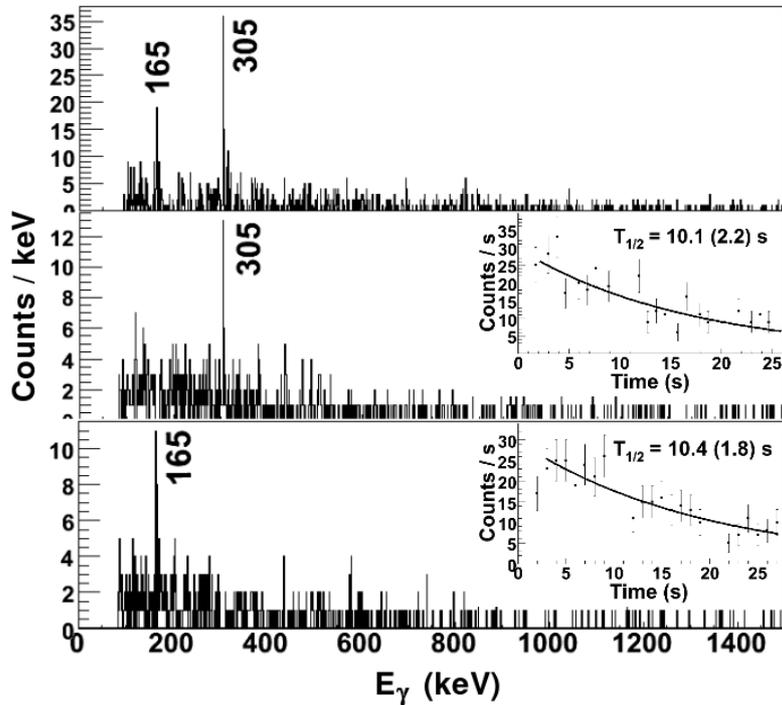
Fig. 2. Upper panel:  $\beta$ -delayed  $\gamma$ -ray spectrum for the  $^{204}\text{Pt} \rightarrow ^{204}\text{Au}$  decay. Middle and bottom panels:  $\gamma\gamma$  coincidences and lifetime curves for the  $\gamma$ -ray transitions of  $^{204}\text{Au}$ .
