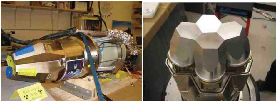
Fig. 6. GRETINA quad module showing the 4 canisters inside the cryostat.
