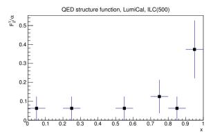
Fig. 4. The QED structure function of a photon divided by the fine structure constant as function of x variable for the mean value of  $Q^2$  equal to 119 GeV<sup>2</sup> (reconstruction level). Only statistical uncertainties are presented.
