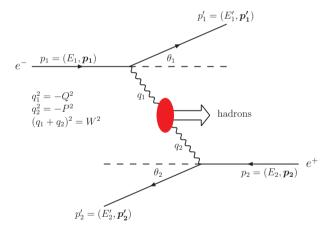
Fig. 1. Kinematics of the two photon process [5].
