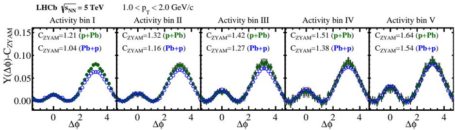
Fig. 3. (Colour on-line) One-dimensional correlation yield as a function of  $\Delta\phi$  for common absolute activity classes in  $p$ -Pb (full/green dots) and Pb- $p$  (open/blue circles) collisions. Figure is taken from Ref. [22].
