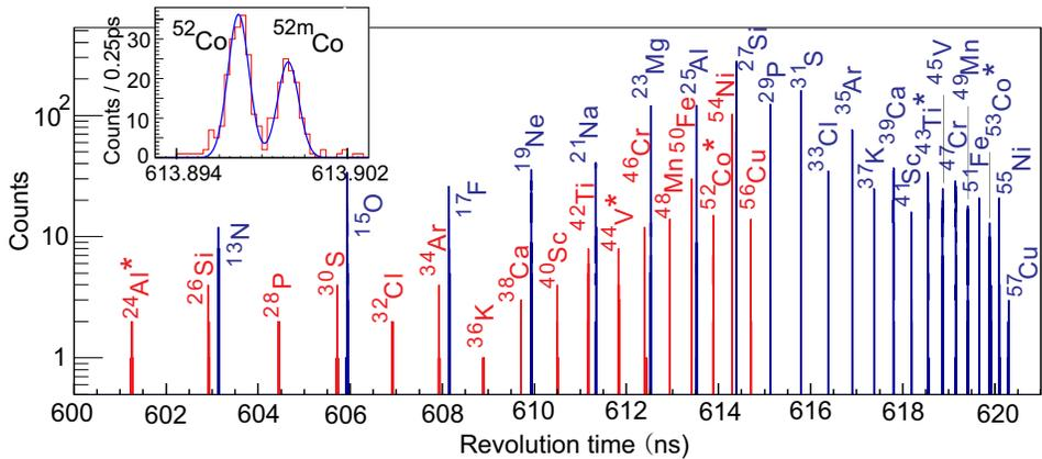
Fig. 1. (Colour on-line) Part of the revolution time spectrum zoomed on the time window of  $600 \text{ ns} \leq t \leq 620 \text{ ns}$ . The light grey/red and dark grey/blue peaks represent the  $T_z = -1$  and  $-1/2$  nuclei, respectively. The asterisks mean that the corresponding peak contains contributions from both ground and isomeric states. The insert shows the well-resolved peaks of the ground and ( $2^+$ ) isomeric states of  $^{52}\text{Co}$ .
