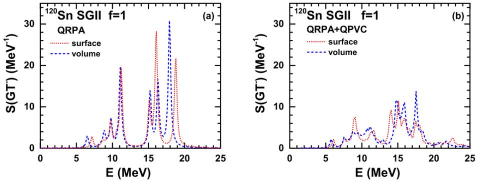
Fig. 1. Gamow–Teller strength distribution in  $^{120}\text{Sn}$  calculated in the QRPA [panel (a)] and in the QRPA+QPVC [panel (b)] model with volume and surface pairing, using the Skyrme interaction SGII.
