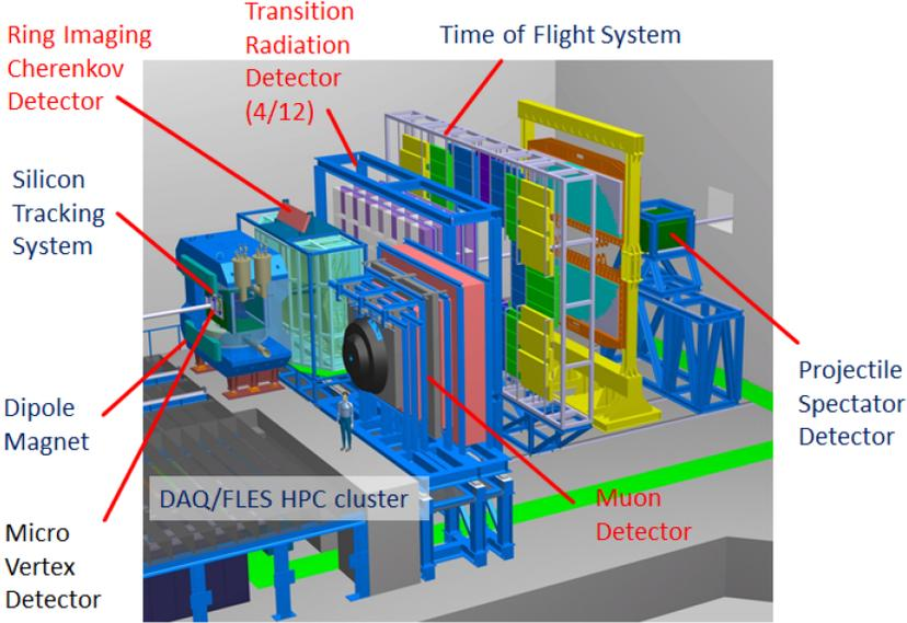
Fig. 2. The CBM experiment in SIS-100 configuration.
