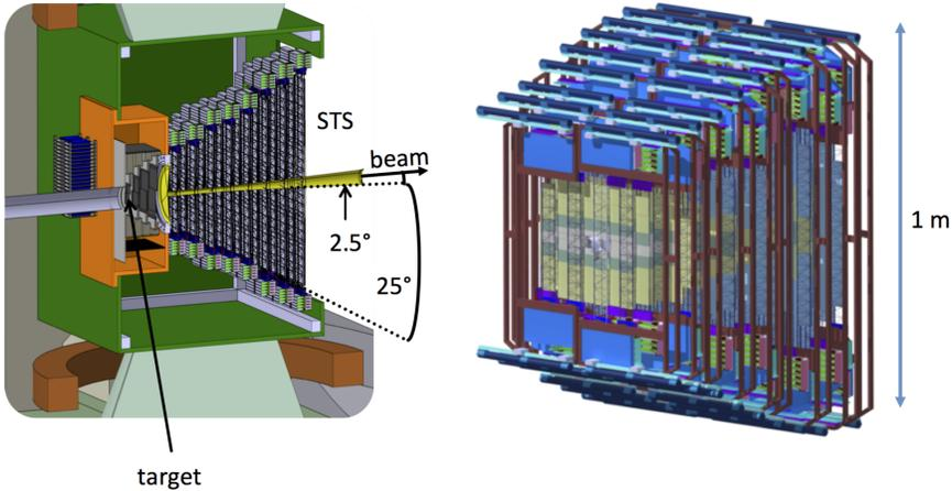
Fig. 3. Engineering views of the Silicon Tracking System.
