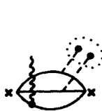
Fig. 11. The simplest quark loop contributing to the polarization operator in external field. Here (and in the following figures) solid lines — quark propagators, dashed lines — gluon propagators, wavy lines correspond to electromagnetic field
