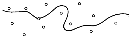
Fig. 3. Example of weakly pinned dislocation loop. Pinners are represented by circles.
