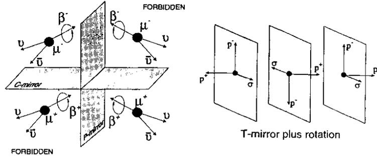
Fig. 1. Discrete transformations. a —  $P$  and  $C$  reflection, b — time reversal in case of pair creation with momenta  $p^-$  and  $p^+$  and spin  $\sigma^-$  of the electron. Followed by a trivial rotation only one of the three vectors remains inverted. TRI assigns equal probability to both orthogonal combinations.
