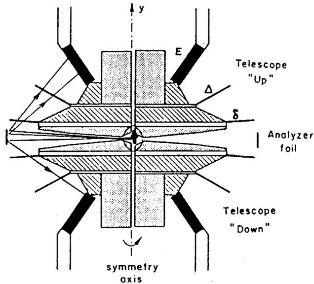
Fig. 6. Ring-shaped Mott polarimeter at ETH-Zurich around  ${}^8\text{Li}^+$  (arrow at center) to test TRI via the  $R$ -term in Eq. (1).
