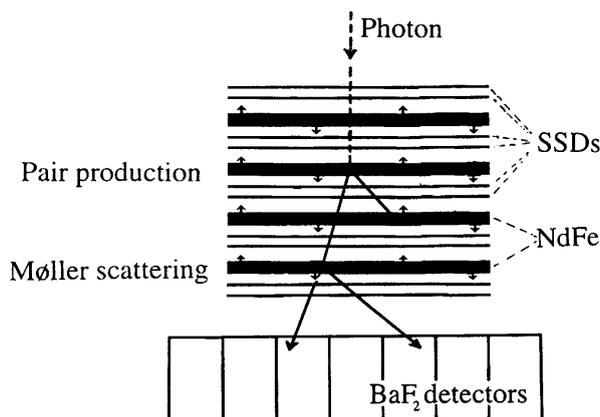
Fig. 7. A concept for polarimetry at energies up to 100 MeV using multiple NdFe + SSD layers. Arrows symbolize the magnetization of the NdFe layers (with chessboard pattern when seen from above).  $\text{BaF}_2$  detectors are added to reconstruct the full energy of the incident photons or leptons.
