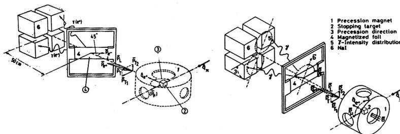
Fig. 4. Longitudinal (left) and transverse (right) polarimetry at PSI with  $\beta^+$  rays from decaying polarized muons.
