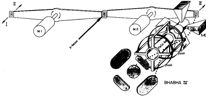
Fig. 3. Fourfold Bhabha polarimetry with fourth polarimeter in detail.
