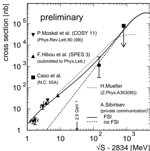
Fig. 5.  $pp \rightarrow pp\eta'$  cross-section as a function of the energy above threshold. DISTO's result (solid circle) is plotted together with threshold measurements and two model calculations underlining the importance of final state interactions (FSI). DISTO's other data taking energy, filling the gap between threshold and the present 144 MeV point, is indicated by the arrow.
