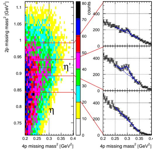
Fig. 4. Left: Correlation of the 4-particle ( $pp\pi^+\pi^-$ ) missing mass and 2-particle ( $pp$ ) missing mass for events with four charged particles ( $pp\pi^+\pi^-$ ) in the final state. Right: Projection of the left figure with respect to the three different gates on the 2-particle missing mass. The  $\eta$  signal in the 4-particle missing mass is only visible when selecting on the  $\eta'$  in the 2-particle missing mass distribution.
