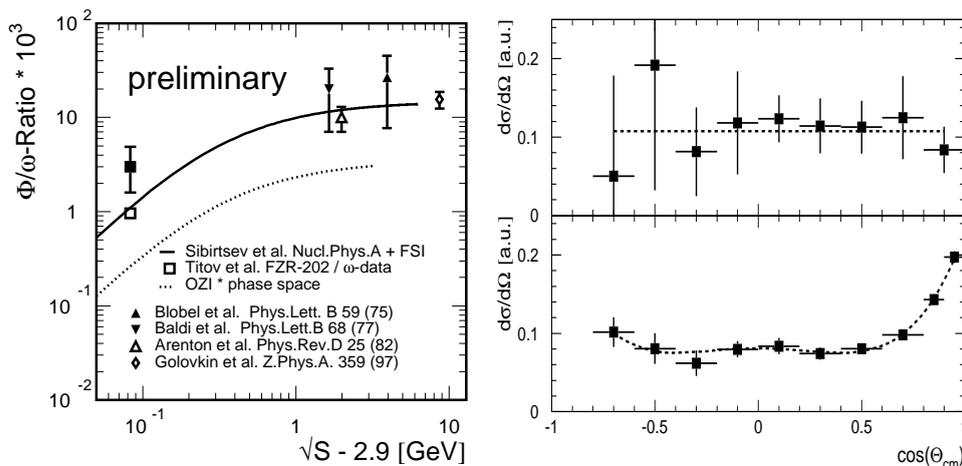
Fig. 3. Left:  $\phi/\omega$  cross-section ratio in  $pp$  collision as a function of the energy above threshold. DISTO's preliminary value at 83 MeV (solid square) is compared to higher energy results, OZI prediction neglecting spin degrees of freedom and model calculations. Right: Angular distributions of the  $\phi$  (top) and  $\omega$  (bottom) mesons, fitted by Legendre expansions.
