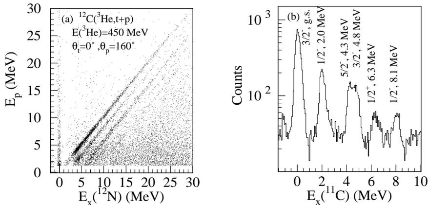
Fig. 1. (a) — two-dimensional scatter plot of proton-triton coincidence events induced by the  $^{12}\text{C}(^3\text{He}, t)$  reaction at  $\theta \sim 0^\circ$ . The loci indicate proton decay to final states in  $^{11}\text{C}$ . Proton events with energies lower than  $\sim 1.2$  MeV are cut off by an electronic threshold. (b) — the final-state spectrum of  $^{11}\text{C}$  obtained by projecting loci in the scatter plot onto the excitation energy axis of  $^{11}\text{C}$ .
