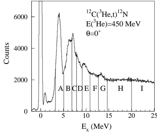
Fig. 3. A singles spectrum at  $\theta = 0^\circ$  for the  $^{12}\text{C}(^3\text{He},t)^{12}\text{N}$  reaction at  $E(^3\text{He})=450$  MeV. The regions denoted as A–I indicate the gating bins for which angular-correlation patterns for proton decay into the final states in  $^{11}\text{C}$  have been determined.
