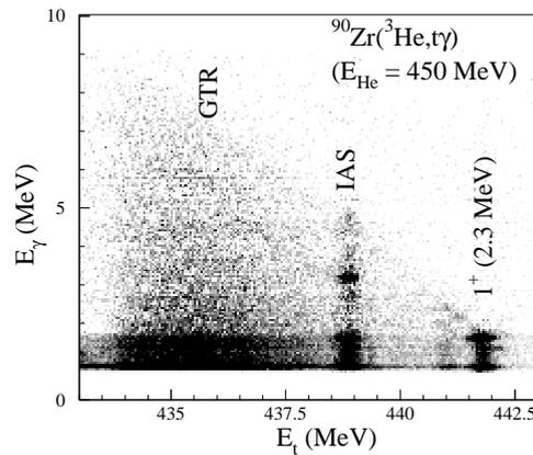
Fig. 2. Two-dimensional scatter plot of  $\gamma$ -ray energy versus triton energy obtained at  $E(^3\text{He}) = 450$  MeV and  $\theta_t = 0^\circ$  is shown for the excitation energy region below the neutron decay threshold in  $^{90}\text{Nb}$  and after unfolding the response of the NaI detectors. The loci for  $\gamma$  decay to the  $2^+$  state at 0.85 MeV and  $1^+$  state at 2.3 MeV are visible.
