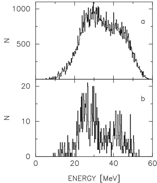
Fig. 2. Energy distribution of all the 2p2h states generated by the six major mean field shells (a). (b) corresponds to those 2p2h states (2) which fulfil the condition  $|\langle 1|\hat{H}|2\rangle| \geq 0.3$  MeV. The symbol N denotes the number of states in the bin of energy equal to 0.2 MeV.
