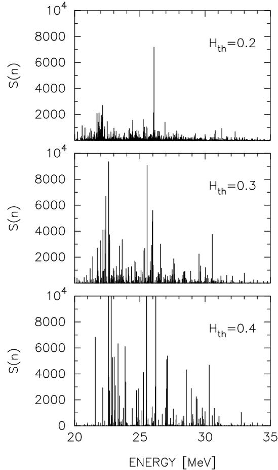
Fig. 4. Isoscalar  $3\hbar\omega$  dipole strength distribution in  $^{208}\text{Pb}$  calculated in the space of 1p1h and 2p2h states, for three different values of  $H_{\text{th}}$ .
