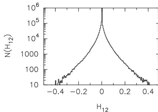
Fig. 1. Distribution of the coupling matrix elements between the 1p1h and 2p2h states for  $J^\pi = 1^-$  sector in  $^{208}\text{Pb}$ .
