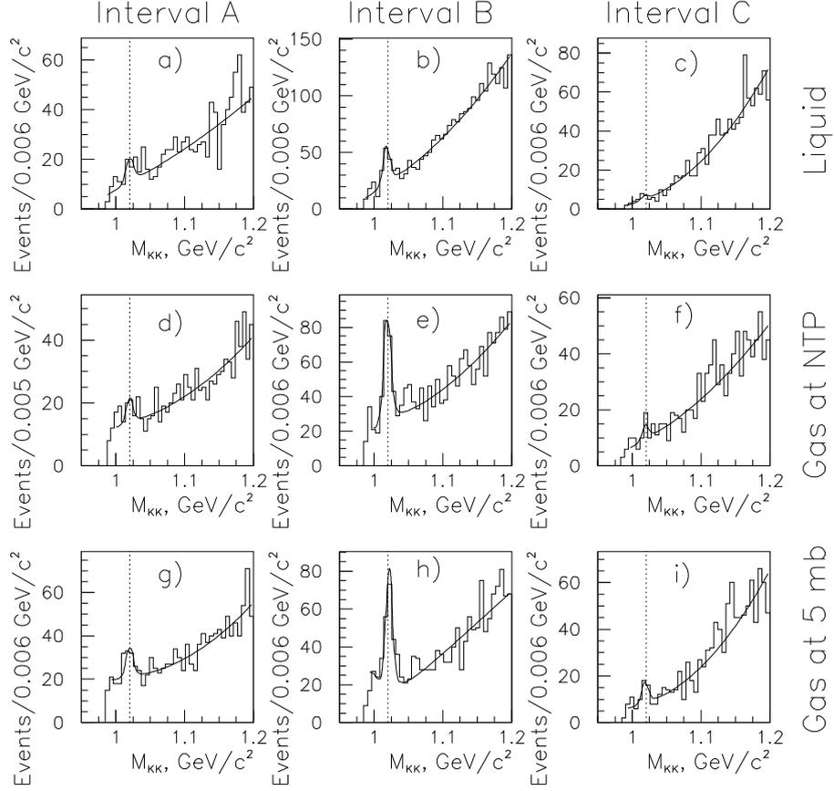
Fig. 1. The distributions on  $M_{K^+K^-}$  for three intervals of missing mass for three target densities: (a), (b), (c) for the liquid target, (d), (e), (f) for the gas target at NTP and (g), (h), (i) for the gas target at 5 mbar. The left column corresponds to central interval (see the text), column (b), (e), (h) corresponds to the left one, and column (c), (f), (i) corresponds to the right one. Dashed lines correspond to the  $\phi$  meson mass.
