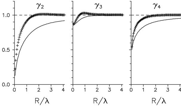
Fig. 1. Friction coefficients  $\gamma_{\text{wall}}^L$  (---),  $\gamma_L$  (+ + +), and  $\gamma_L^{[0]}$  (—) for  $L=2$  (left), 3 (middle), and 4 (right) as functions of the ratio  $R/\lambda$ .
