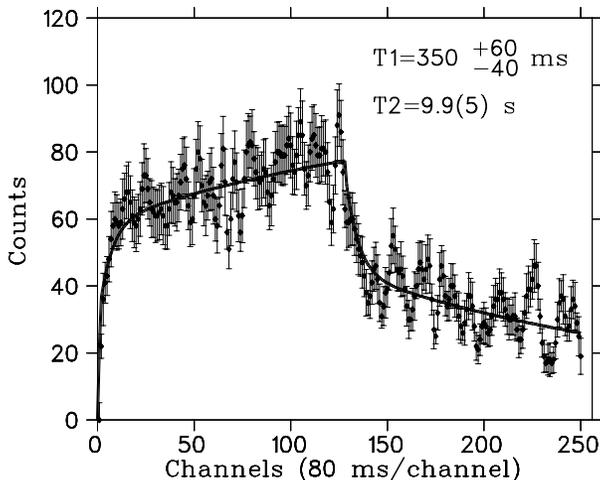
Fig. 2. Growth and decay of singles K+L+M electrons of the 107.0 keV E3 transition. The curve is calculated with two components + long-lived contamination.
