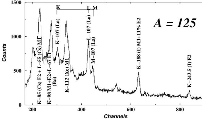
Fig. 1. Partial conversion electron spectrum measured with the ELLI spectrometer.
