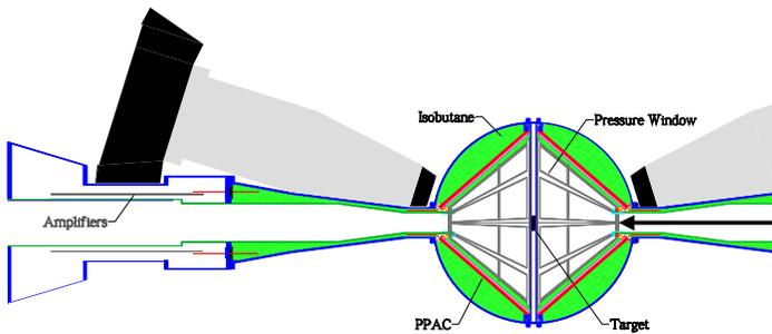
Fig. 1. Schematic of the PPAC array CHICO and two representative Gammasphere Ge detectors.
