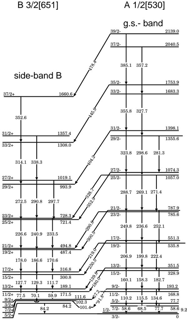
Fig. 2. Proposed levels and their assignment to the known bands in  $^{231}\text{Pa}$  according to observed particle- $\gamma$ -coincidences.
