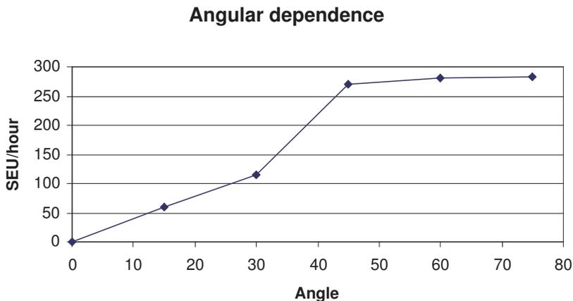
Fig. 3. Number of SEUs as a function of the beam incident angle to the chip
