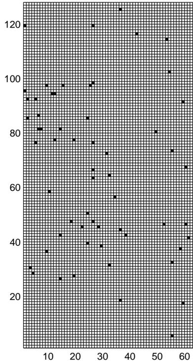
Fig. 2. Virtual memory map. The black areas are the memory cells, where temporary errors of Single Event Upset type were detected during irradiation.
