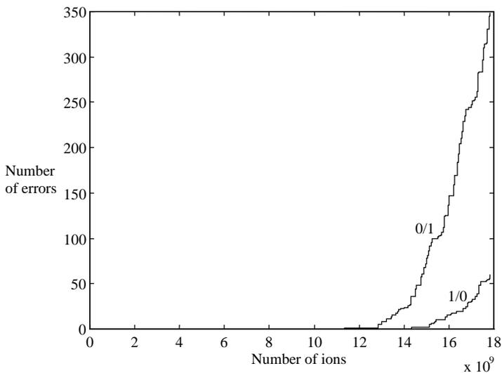
Fig. 4. Number of errors as a function of incident particles
