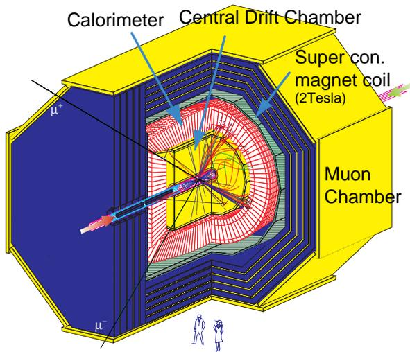
Fig. 2. Schematic view of the JLC detector. The total volume is  $16 \times 16 \times 16\text{m}^3$ , and it weighs 15,000 tons. Superimposed is a Higgs boson production event at  $\sqrt{s}=300\text{GeV}$  assuming  $m_h=120\text{GeV}$ , ( $e^+e^- \rightarrow Zh$ ,  $h \rightarrow b\bar{b}$ ,  $Z \rightarrow \mu^+\mu^-$ ) The simulation is based on GEANT3.21.
