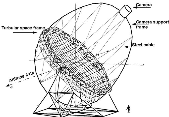
Fig. 7. A model of the 17m  $\odot$  MAGIC telescope.
