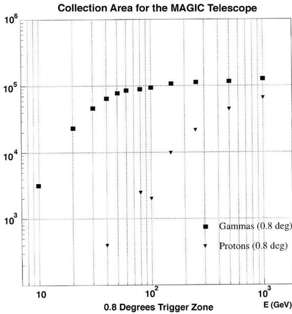
Fig. 8. Collection area as function of  $E$ . In brackets: radius of trigger area.
