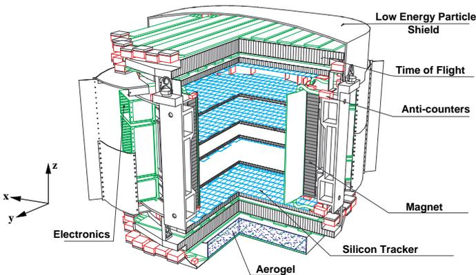
Fig. 2. AMS experimental setup for the STS-91 flight
