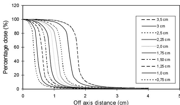
Fig. 2. Beam profiles (OAR) of 6 MeV X-ray beam formed with collimators of 0.75 cm to 3.00 cm in diameter, measured with diamond detector.
