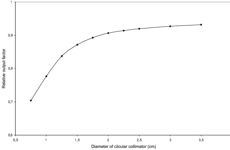
Fig. 3. Relative output factors (ROF) of 6 MeV X-ray beam formed with collimators of 0.75 cm to 3.0 cm in diameter and with primary jaws field size setting  $5 \times 5 \text{ cm}^2$ , measured using ion chamber.
