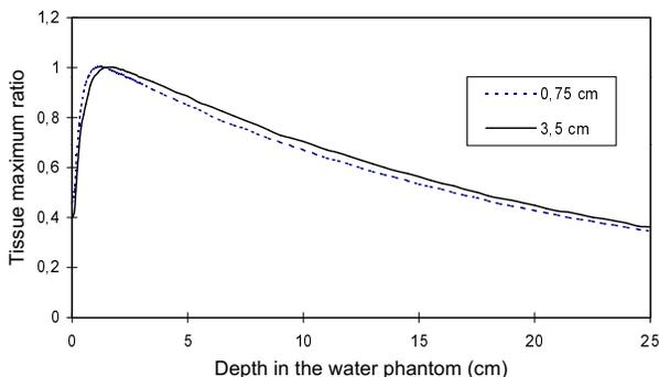
Fig. 1. Tissue maximum ratio (TMR) of 6 MeV X-ray beam, measured for 0.75 cm and 3.50 cm collimator diameters using 0.015 cm<sup>3</sup> ion chamber.
