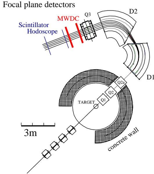
Fig. 2. Schematic view of BIG KARL magnetic spectrometer consisting of three quadrupoles Q1, Q2 and Q2a and two dipoles D1 and D2. The quadrupole Q3 was not used. The particles could be measured by means of the detectors at the focal plane: two layers of scintillator hodoscope and two stacks of Multi-Wire Drift Chambers (MWDC).
