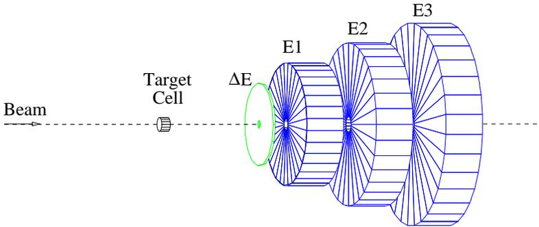
Fig. 1. Schematic view of Germanium Wall detector. All the set-up has a radial symmetry. The first element denoted by  $\Delta E$  has a structure of 200 Archimedes spirals with right or left orientation depending on the detector side. Other elements denoted by  $E$  consist of 32 wedges.
