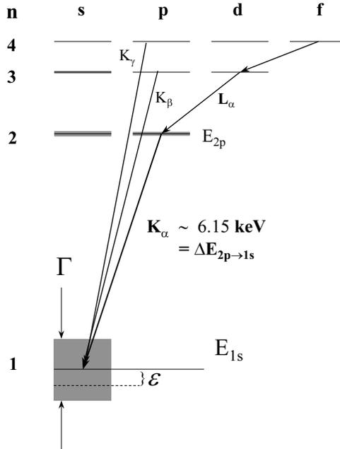
Fig. 1. Schematic view of the level scheme of kaonic hydrogen indicating the  $K_\alpha$ ,  $K_\beta$  and  $K_\gamma$  transitions, and the level shifts and widths, which are only relevant for states  $n \leq 2$ .
