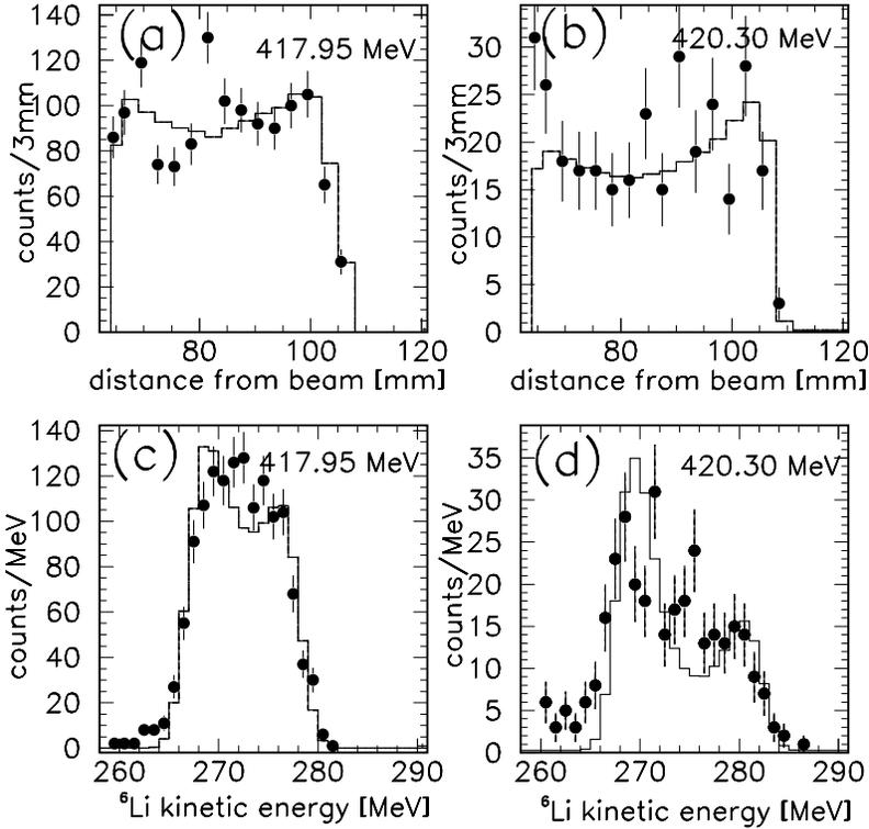
Fig. 1. Position and energy spectra. The filled circles represent experimental data and the histograms results from the fits described in the text. Top: horizontal position distributions for (a) 417.95 MeV and (b) 420.30 MeV. Bottom: energy spectra for (c) 417.95 MeV and (d) 420.30 MeV. For (d) events with energies between 266 and 286 MeV were included in the fit.
