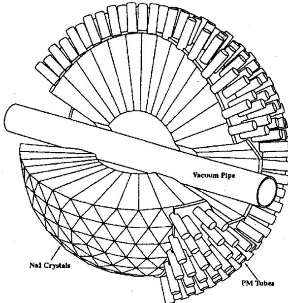
Fig. 1. Geometry of the Crystal Ball. Not shown are the 10 cm long liquid hydrogen target in the center and the 1.2 m long veto barrel which surround the target and vacuum pipe.
