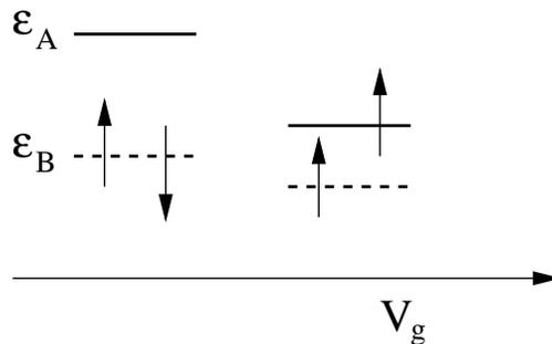
Fig. 1. The relative distance between  $\varepsilon_A$  and  $\varepsilon_B$  levels changes when the non-uniform gate potential  $V_g$  increases. If  $\varepsilon_A - \varepsilon_B > J$  then the lower  $\varepsilon_B$  level is doubly occupied and the total spin is zero. However, when  $\varepsilon_A - \varepsilon_B < J$  then the two levels are single occupied and the total spin is one.
