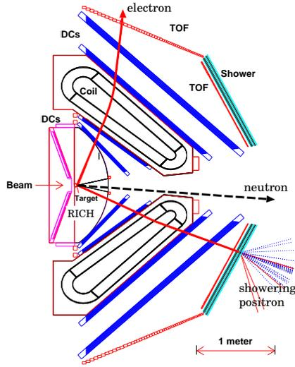
Fig. 16. Schematic diagram of the dilepton spectrometer HADES.
