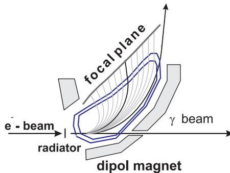
Fig. 3. Energy tagging of bremsstrahlung photons.
