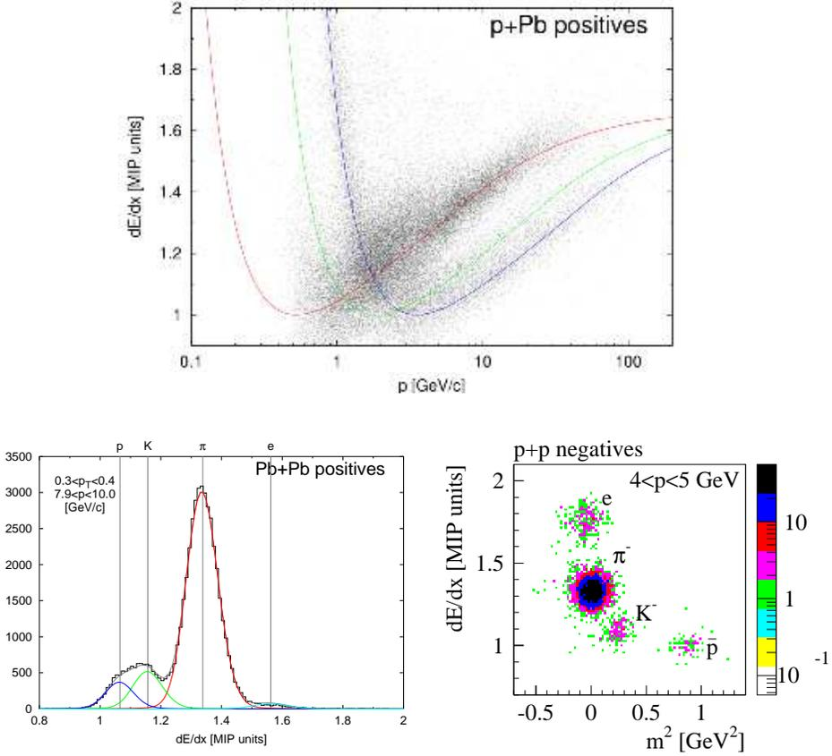
Fig. 4. Particle identification data for nuclear collisions at 158 GeV/c, using ionisation sampling in time projection chambers and time of flight measurements.
