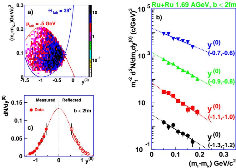
Fig. 1. (a) Phase space distribution of  $K^+$  mesons measured in the experiment  $^{96}\text{Ru}+^{96}\text{Ru}$ . (b) Transverse mass spectra of  $K^+$  mesons in different rapidity slices. Lines depict the fits according to the formula (1). (c) Rapidity density distribution of  $K^+$  mesons. The line depicts the distribution obtained for a thermalized source of temperature  $T=80$  MeV.
