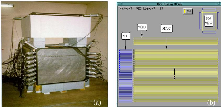
Fig. 1. (a) The modified configuration of the WILLI detector (with anti-counters); (b) Event display: ADC and MTDC image of a muon decay event; the ADC scale corresponds to the 0–4095 channel range and the MTDC comprises 256 bins of 20 ns width; the muon stops after penetrating 6 active layers and the electron appears in the following 3 layers [5].
