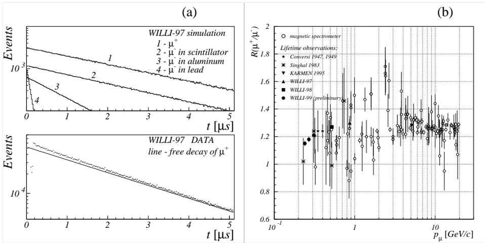
Fig. 2. (a) Monte Carlo simulations results of the contribution of different materials to the total decay curve and the experimental decay curve compared with the decay curve expected for positive muons [7]. (b) The present experimental knowledge of muon charge ratio.
