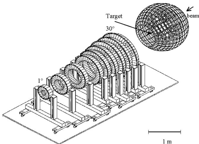
Fig. 1. Isometric drawing of the CHIMERA multidetector
