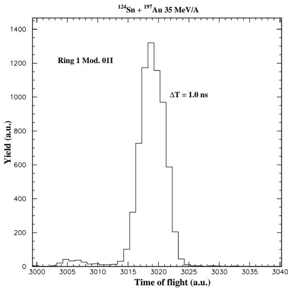
Fig. 12. Elastic peak time resolution measured for the reaction Sn+Au at 35 MeV/A.
