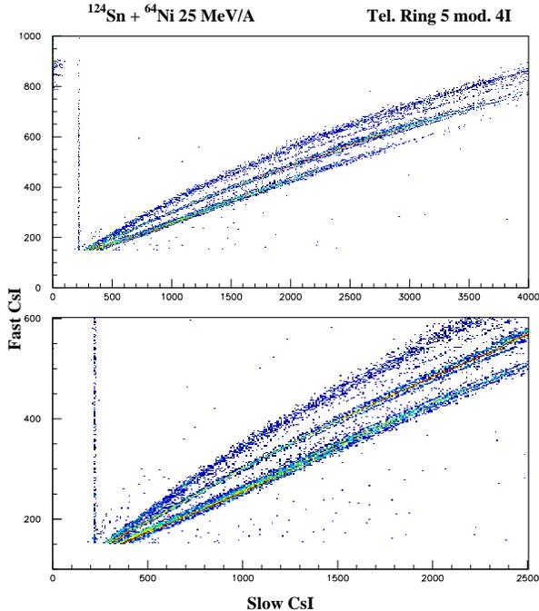
Fig. 14. Isotopic identification of light charged particles (LCP) in the CsI(Tl) detector by using the pulse shape method of the photodiode signal, in the first run of REVERSE experiment,  $^{124}\text{Sn}+^{64}\text{Ni}$  at 25 MeV/A carried out at LNS. Lower side is a zoom of the upper side.
