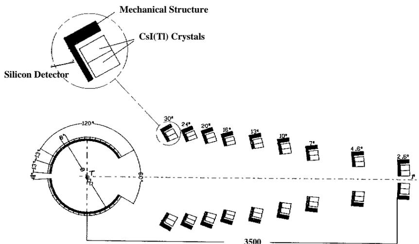
Fig. 2. Cross section drawing of CHIMERA. The number of telescopes placed in 9 wheels between  $1^\circ$  and  $30^\circ$  is 688. The remaining 504 telescopes are placed in a spherical configuration around the target.
