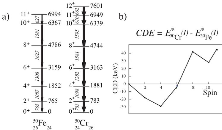
Fig. 5. Comparison of the g.s. bands (a) and the Coulomb difference energies (b) for the  $A = 50$  mirrors  $^{50}\text{Cr}$  and  $^{50}\text{Fe}$ .
