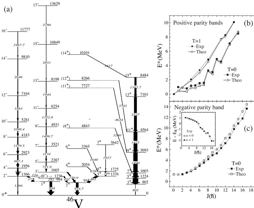
Fig. 4. Level scheme (a) and the experimental excitation energy vs. spin plot for the positive (b) and negative (c) parity bands of  $^{46}\text{V}$  (black symbols) compared with shell model calculations from Ref. [12] (open symbols)
