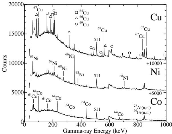
Fig. 2. Gamma-ray spectra measured with the isomer-scope. They were obtained from  $\Delta E$ - $E$ - $\gamma$  coincidence data by setting windows on the  $\Delta E$ - $E$  plot for Cu, Ni, and Co isotopes, respectively.
