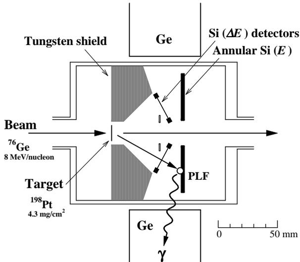
Fig. 1. Isomer-scope: an experimental setup to measure  $\gamma$  rays from isomers with  $T_{1/2} > 1$  ns of projectile-like fragments produced in deep-inelastic collisions. It consists of an annular-type Si detector working as a stopper of PLFs, four Si  $\Delta E$  detectors, four Ge detectors, and a tungsten block to absorb prompt  $\gamma$  rays emitted at the target.
