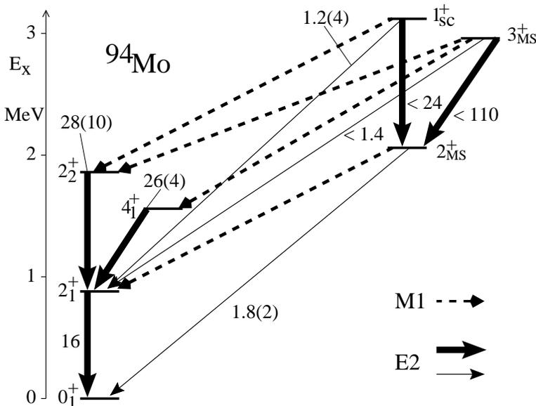
Fig. 1. Partial level scheme of  $^{94}\text{Mo}$  (from [13]). The numbers denote  $B(E2)$  values in Weisskopf units. For  $B(M1)$  values see Table I.
