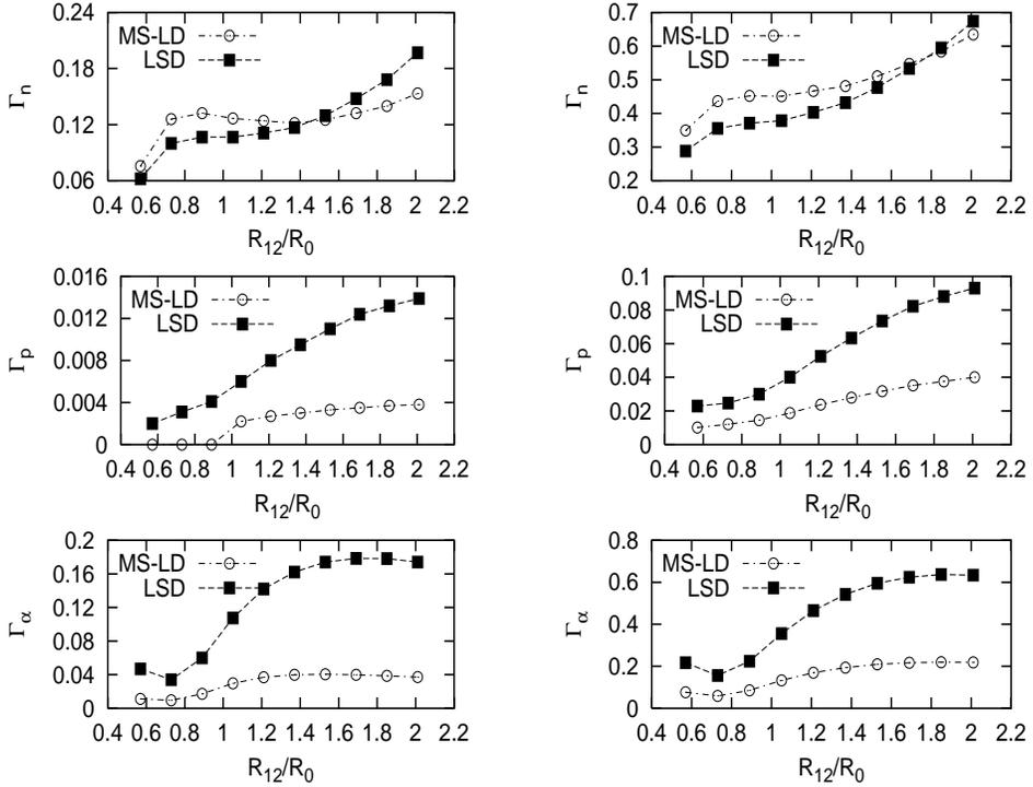
Fig. 1. Neutron, proton and  $\alpha$  particle emission widths  $\Gamma_n$ ,  $\Gamma_p$ ,  $\Gamma_\alpha$  as a function of nuclear elongation  $q = R_{12}/R_0$  for the compound nucleus  $^{188}\text{Pt}$  at an angular momentum  $L = 60\hbar$  and an excitation energy  $E^* = 60$  MeV (left side) and  $E^* = 100$  MeV (right side).
