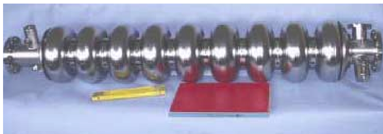
Fig. 1. Photo of a TESLA 9-cell Nb cavity.
