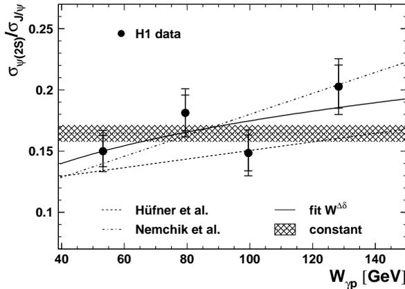
Fig. 1. The ratio  $R(W_{\gamma p}) = \sigma_{\psi(2S)}/\sigma_{J/\psi}$  for events with  $z > 0.95$ . The inner error bars show the statistical error, the outer error bars show the statistical and systematic errors added in quadrature. The result of a fit  $R \propto (W_{\gamma p}/90 \text{ GeV})^{\Delta\delta}$  is shown by the solid line and the predictions from [2] (dashed-dotted line) and [1] (dashed line) are also shown.
