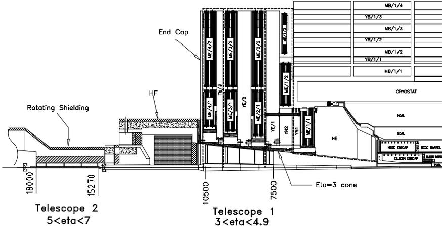
Fig. 1. Position of the inelastic event tagging detectors of TOTEM, T1 and T2, integrated with CMS.
