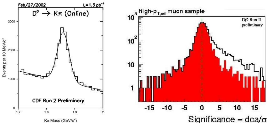
Fig. 3.  $b$ -tagging capabilities. Charm mass peak from CDF (left) and signed impact parameter plot from DØ.
