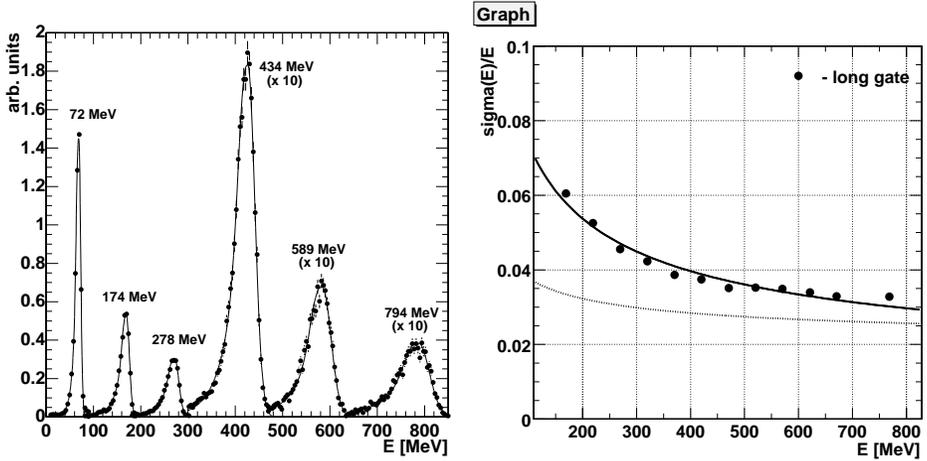
Fig. 2. Left: Experimental line-shapes for various incident photon energies determined in the detector array and recorded with the new electronics. Right: Energy resolution of the BaF<sub>2</sub>-matrix measured for the long integration gate as a function of incident photon energy.
