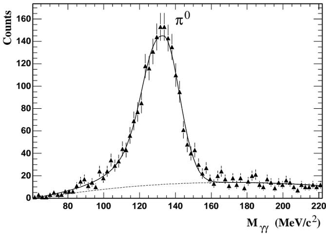
Fig. 3. Invariant mass spectrum deduced from  $\gamma\gamma$ -coincidence detected in the reaction  $\gamma+{}^4\text{He}$  showing a pronounced  $\pi^0$  peak. One of the decay photons was detected in the small detector array read out with the new TAPS electronics. The solid line represents a fit with the known  $\pi^0 \rightarrow \gamma\gamma$  line shape including the combinatorial background (dotted line).
