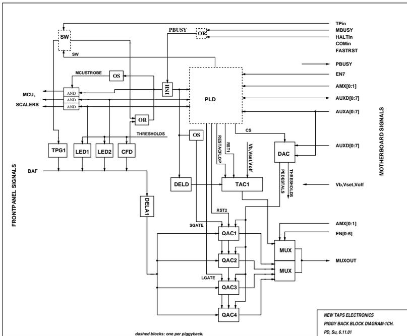
Fig. 1. Schematic block diagram of the piggyback designed for the read out of 4 channels. The upper part shows the digital control circuits for the analogue section (QACs and TAC) below.
