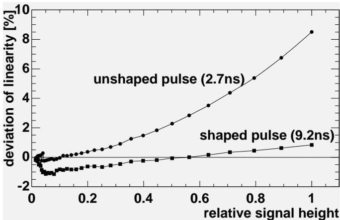
Fig. 4. The measured deviation from linearity shown for an unmodified  $\text{BaF}_2$ -signal (risetime = 2.7 ns) as a function of relative signal amplitude. Maximum values up to 8% have been determined. After shaping leading to an increase of the risetime to 9.2 ns, the maximum non-linearity is reduced down to 1.1%
