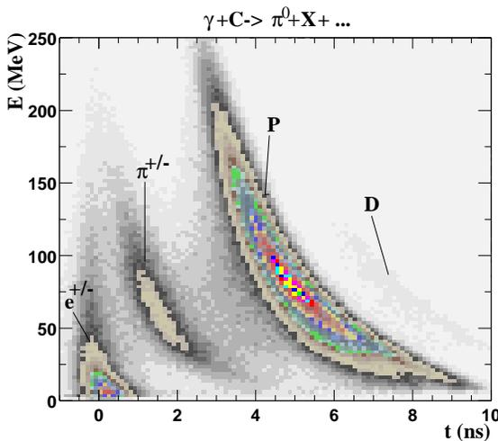
Fig. 3. Energy *versus* time spectrum of charged particles for the reaction  $(\gamma+C \rightarrow \pi^0+X)$  is plotted. The branches of different particles are clearly separated.
